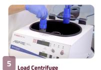
Fill Counterweight with water/saline - ensure same weight as Separator\*
